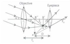
Magnifying power or angular magnification of an astronomical telescope is defined as the ratio of the angle subtended at the eye by the final image at the least distance of distinct vision to the angle subtended at the eye by the object at infinity, when seen directly.
