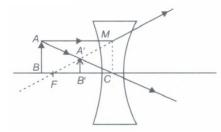
The image formed is virtual, erect and smaller in size.
