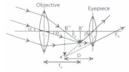
For an astronomical telescope, we will select lens of power 10D for eye piece and lens of power 0.5 D for objective because magnifying power of telescope is  $m = \frac{f_o}{f_c}$
